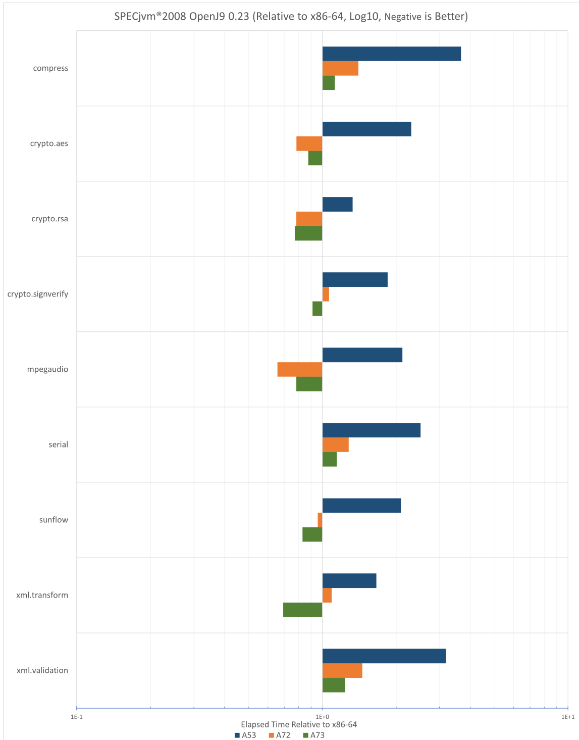
Figure 4.2: SPECjvm ® 2008 elapsed time relative to x86-64 device comparison for OpenJ9 0.23 (Log10, negative is better).
